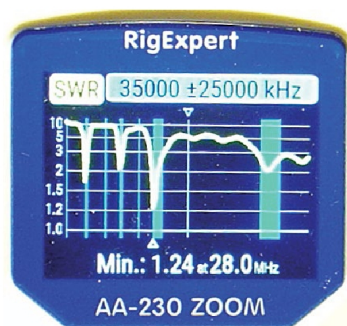
Figure 9 — A 10 – 60 MHz scan of the author's TH1 antenna. Note that the frequency of minimum SWR is indicated.
