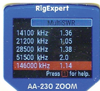
Figure 8 — Using the AA-230 ZOOM's multi-band feature to check the author's TH1 antenna on 20, 15, 10, 6, and 2 meters.
