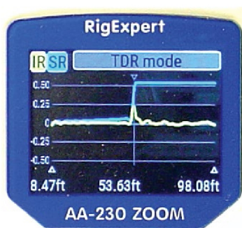
Figure 12 — The AA-230 ZOOM's TDR mode used to find the length of feed line to the author's 43-foot vertical.
