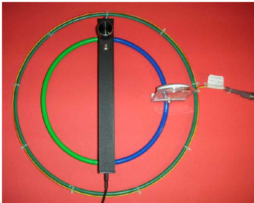
Left and above: Coupling loop for receiver calibration
